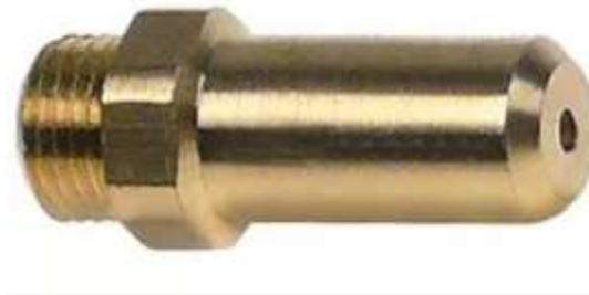
Fig. 5 Boquilla De Gas Rosca M10 X1 Taladro Ø 1,2MM L 30MM EC 12
