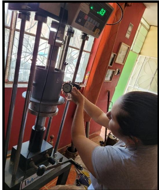
**FOTO 08:** Ensayo California Bearing Ratio (CBR)
