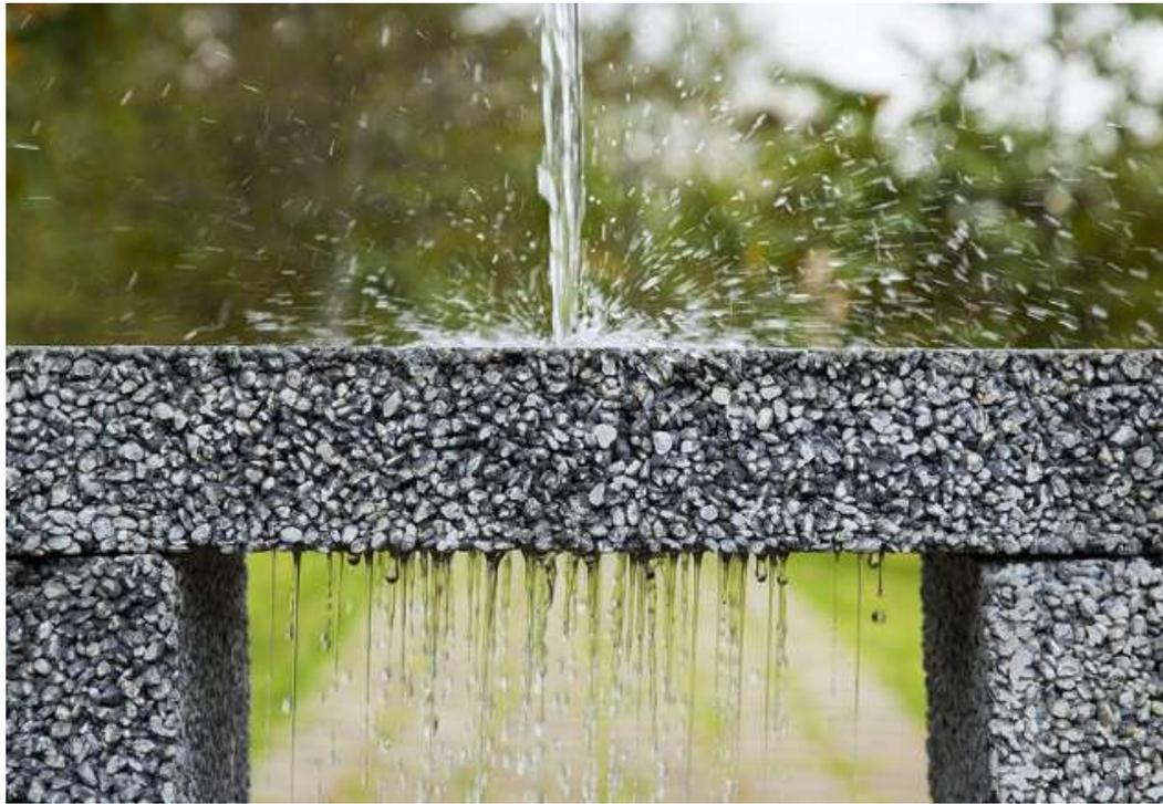
**Figura 19.** Concreto Permeable
